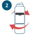
Turn used filter left 1/4 turn to remove from filter head.
